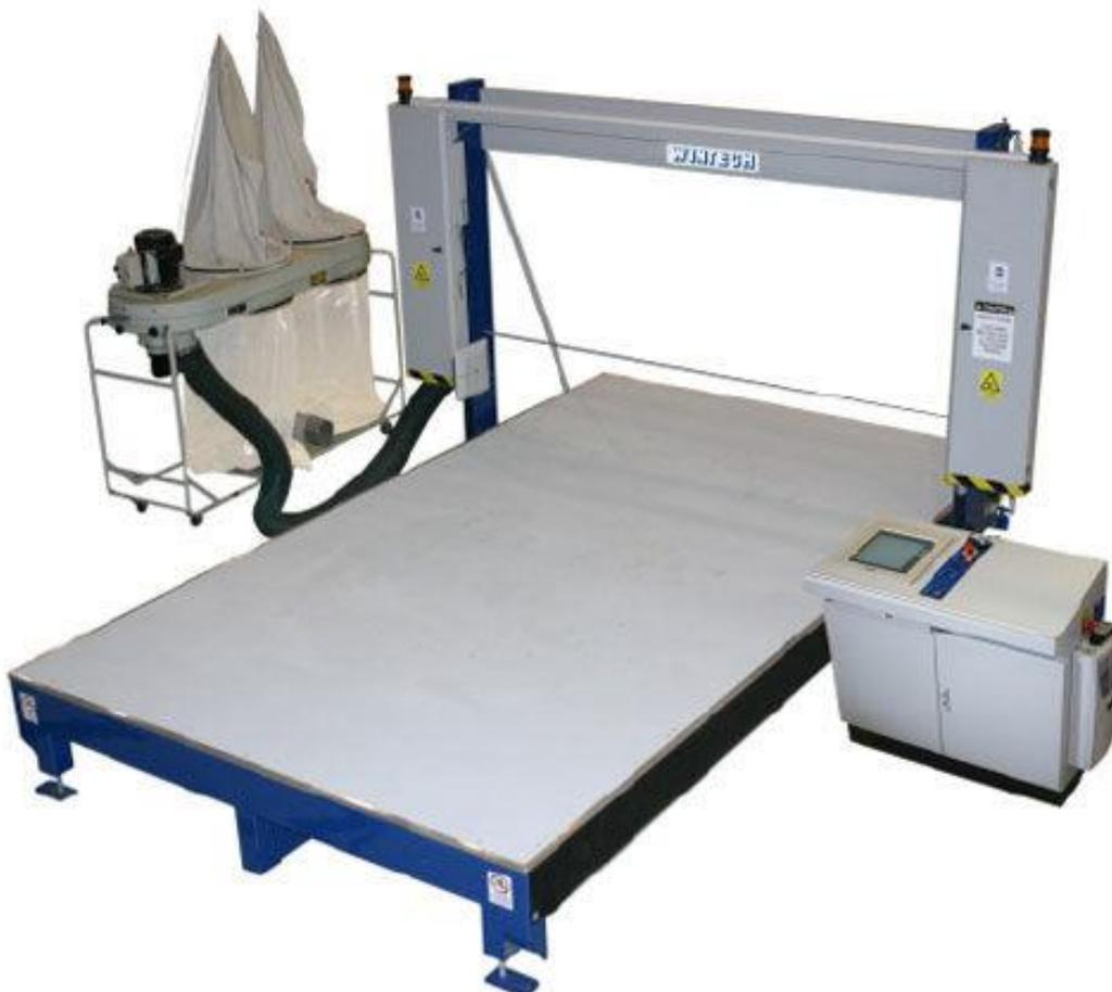
Figura 3. Máquina CNC de corte de hilo. Fuente: <https://www.directindustry.es/prod/wintech-engineering/product-78368-1491599.html>
